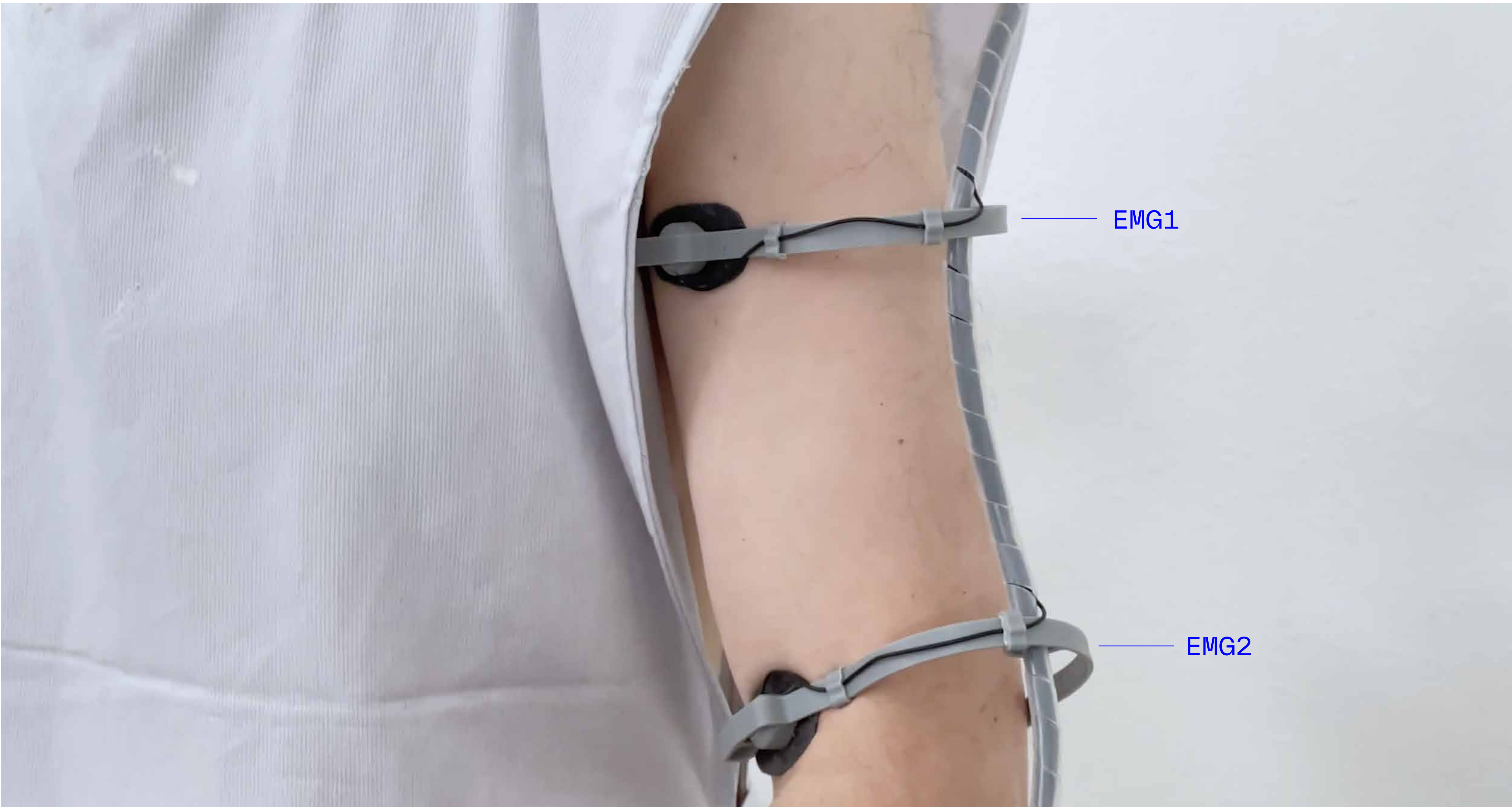
3-Final prototype -EKG, EMG 1 AND EMG2 easy to put on and flexible monomaterials
