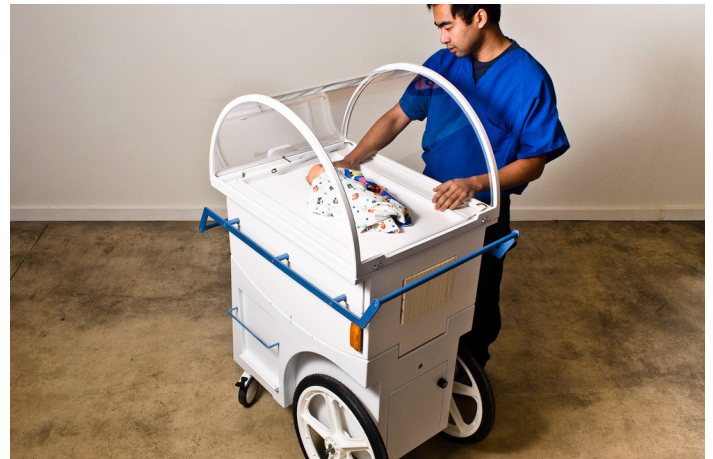
Figure 14: NeoNurture Incubator Designed Using Car Parts
