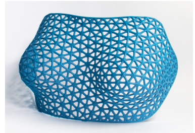
Chest protector prototype in PETG
