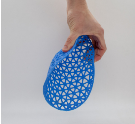
Flexibility of the TPU for AMS lattice prototype
