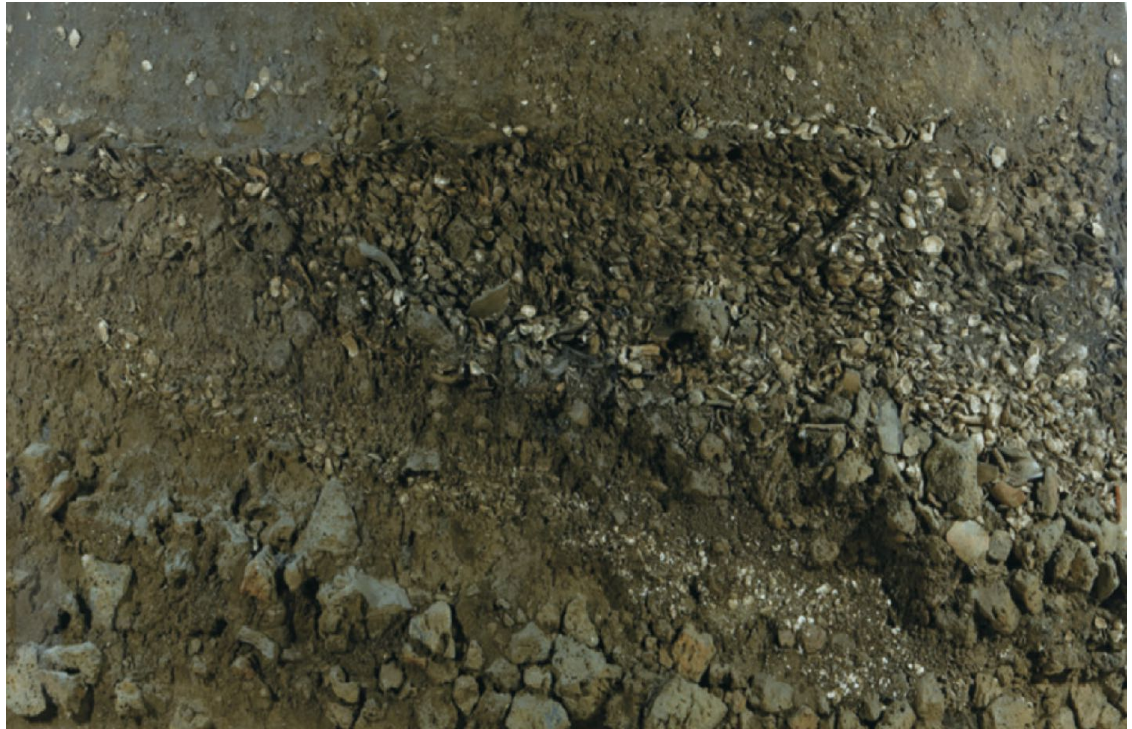
This image shows the soil conditions of Jeju Island. In this area, the ground consists mostly of solid rock, with only small amounts of soil mixed in.
