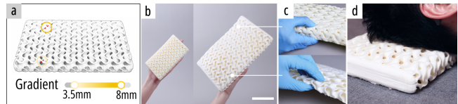
Figure 16: GyFoam pillow: (a) Constructing the pillow with a wall thickness gradient using our design tool; (b) Expanding to a single-person pillow; (c) Varying stiffness between the two sides; (d) Allowing users to rest on the preferred side based on desired firmness. Scale bar: 100 mm.
