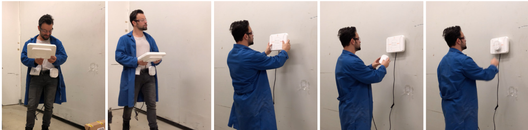
Placing products on the belt Going to the workspace Buried hole scanning Attached the drill to the main body Pressing the button for drilling
