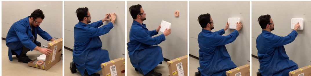
Taking target piece from a box Buried hole scanning and surface locking Taking main body from a box Locking on the target piece. Pressing the button for drilling
