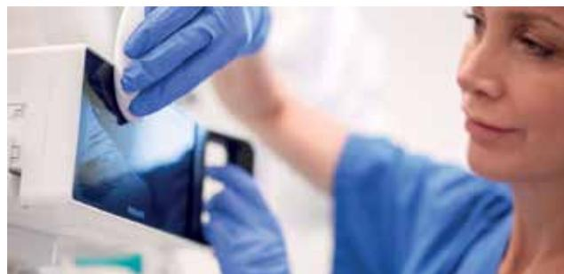
The part of the X3 you touch most often — its touchscreen display — is covered with Antimicrobial Corning® Gorilla® Glass, embedded with an ionic silver with antimicrobial properties that lasts through the lifetime of the touch display.
