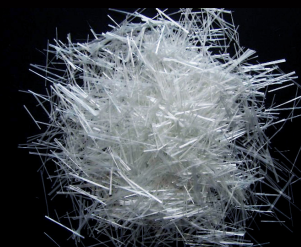
ICE REINFORCEMENT: POLYMER FIBER
