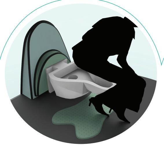
When approaching the toilet, the user turns around and steps on the weight distribution mat. While pressure is put on the mat, the hole that covers the waste opens to allow waste easy passage. When the user steps off of the mat, the hole closes back up. This feature eliminates a touch point, encourages the user to be more respectful to the space and eliminates odors. The seat is also re-designed so that "hovering" is much easier and less messy.
