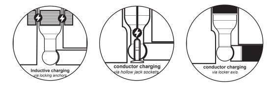
Figure 27: Quickdesigns regarding power transmission from the locker on to the bicycle
