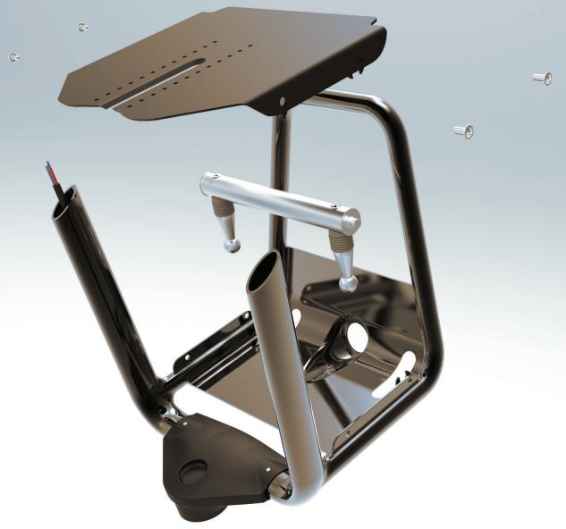
Figure 59 : Cutaway view of the luggage rack
