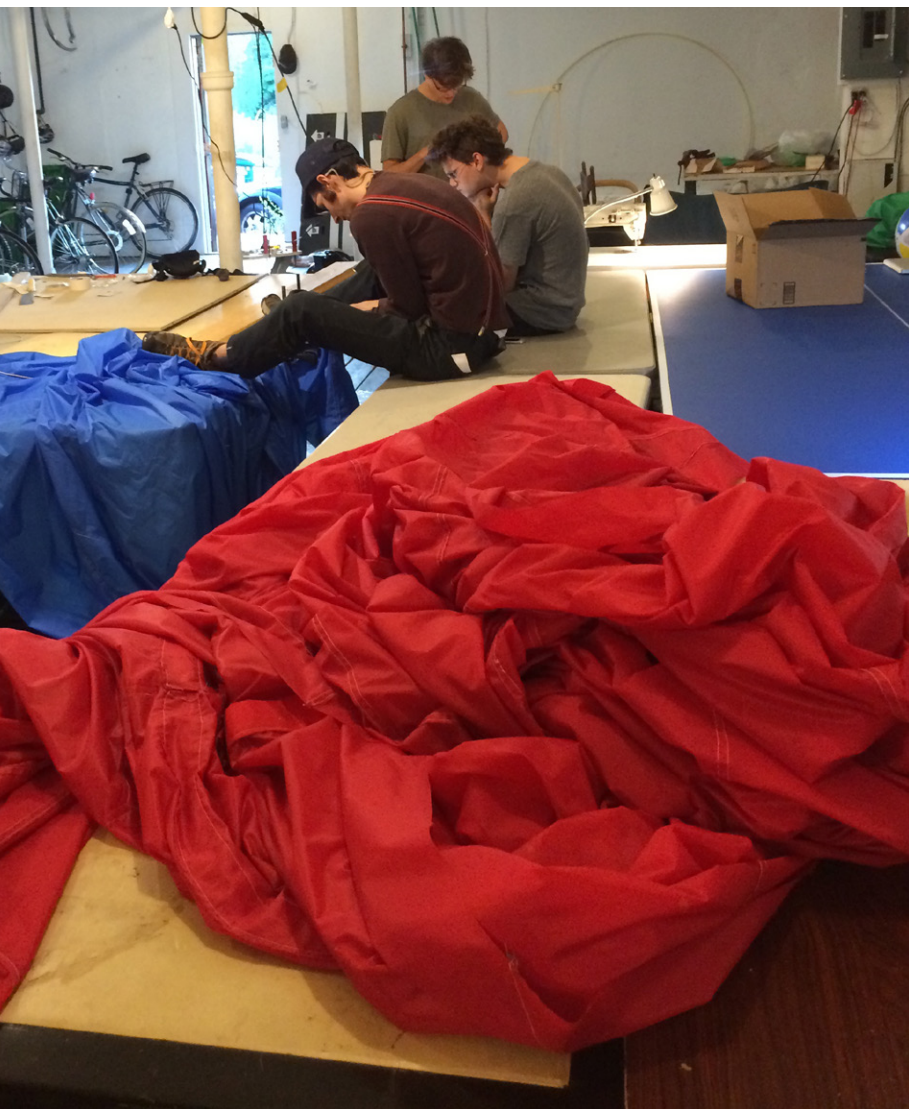
Seams are double-stitched to give strength and a flat surface.
