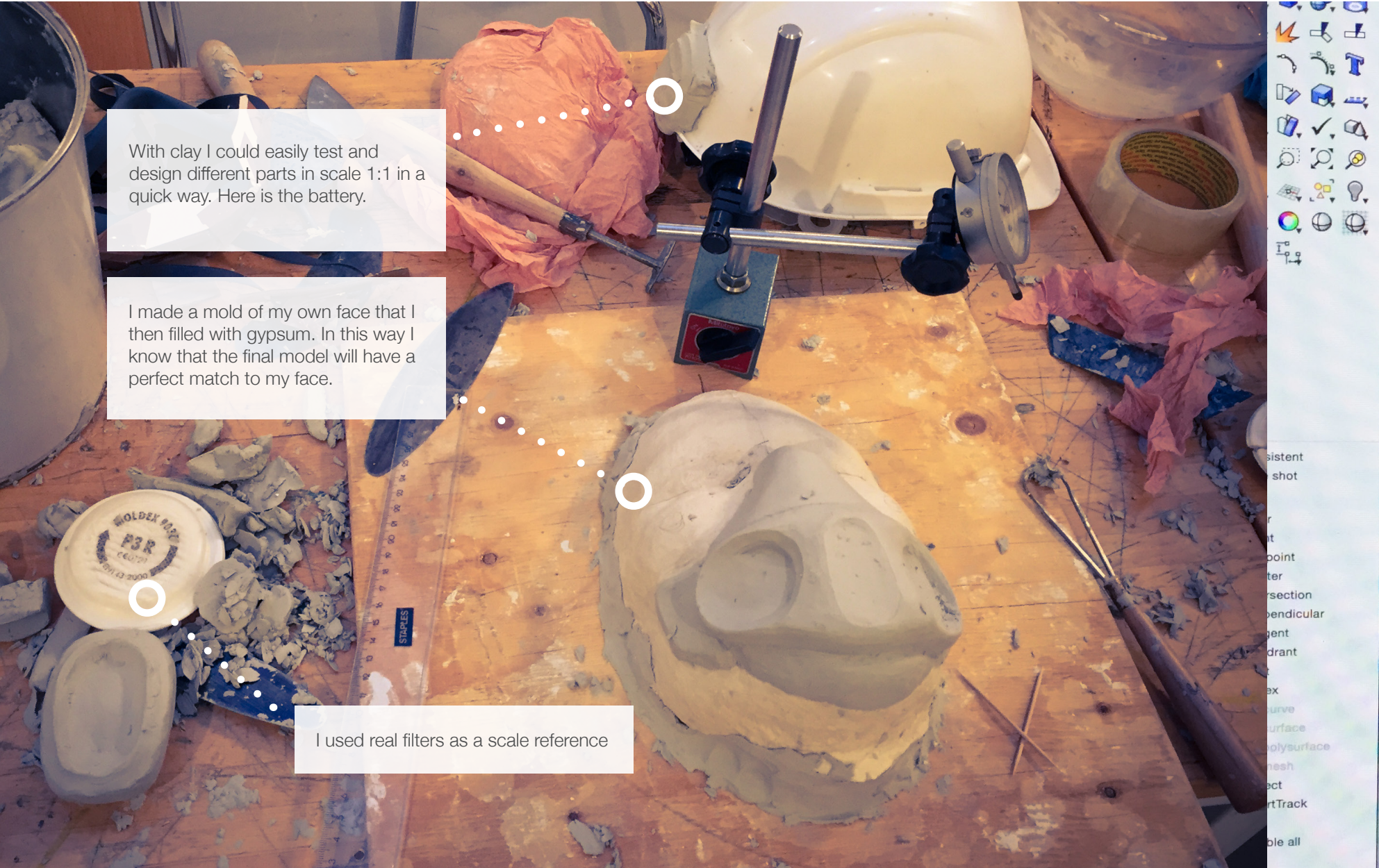
I worked parallel between clay modeling and CAID to explore the shapes and proportions on the different parts. This gave me a fast workflow to a decided design and a finished model.
